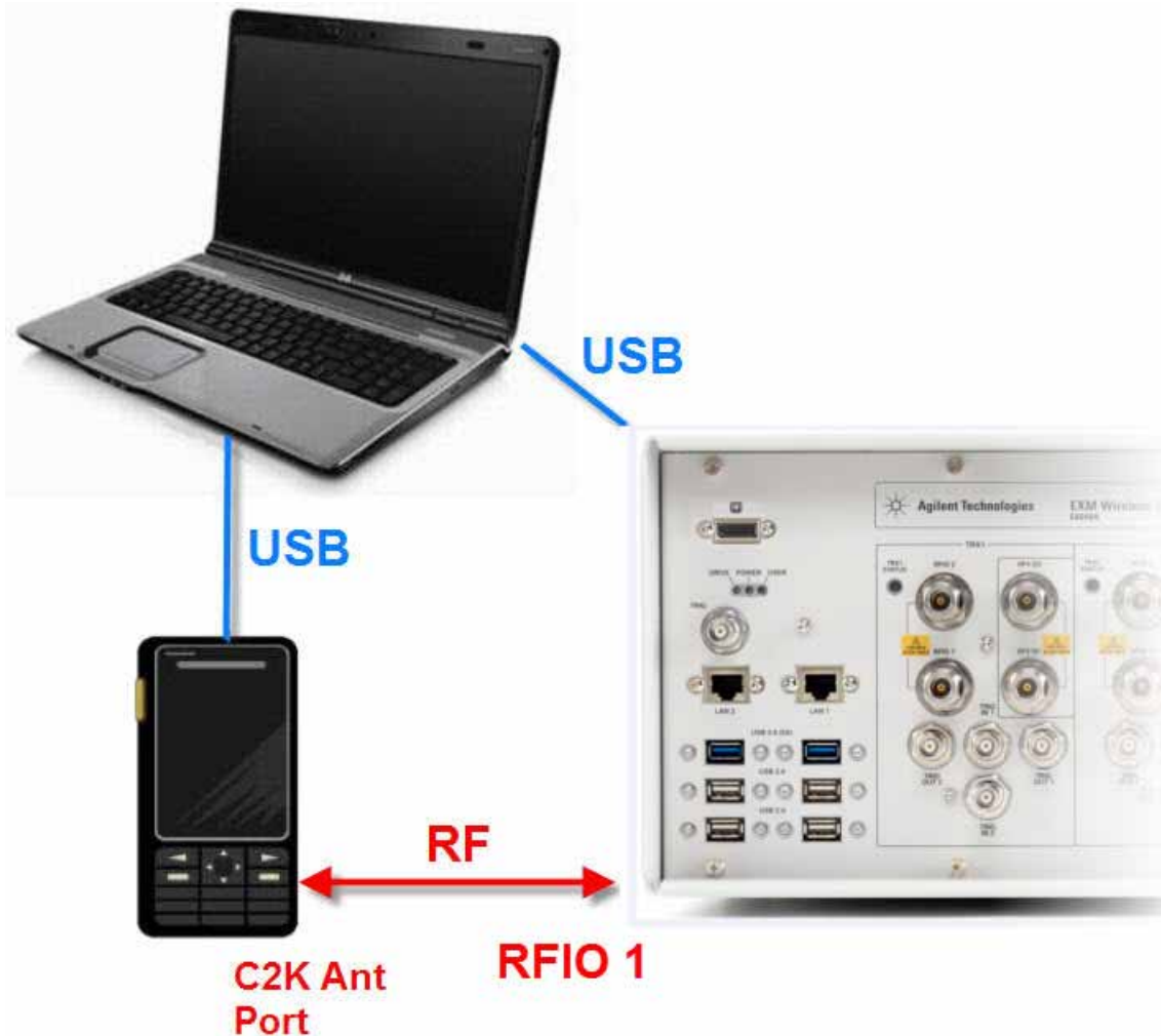
Figure 11-1 Hardware Setup for Calibration Example
